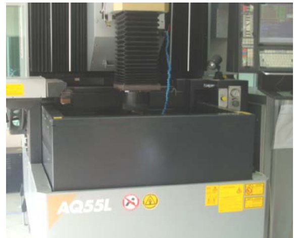
(b) EDM tank with electrode and workpiece.
