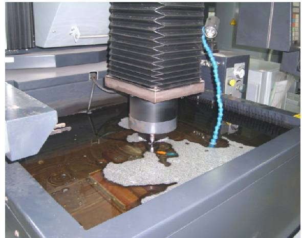
(a) EDM at machining state.
