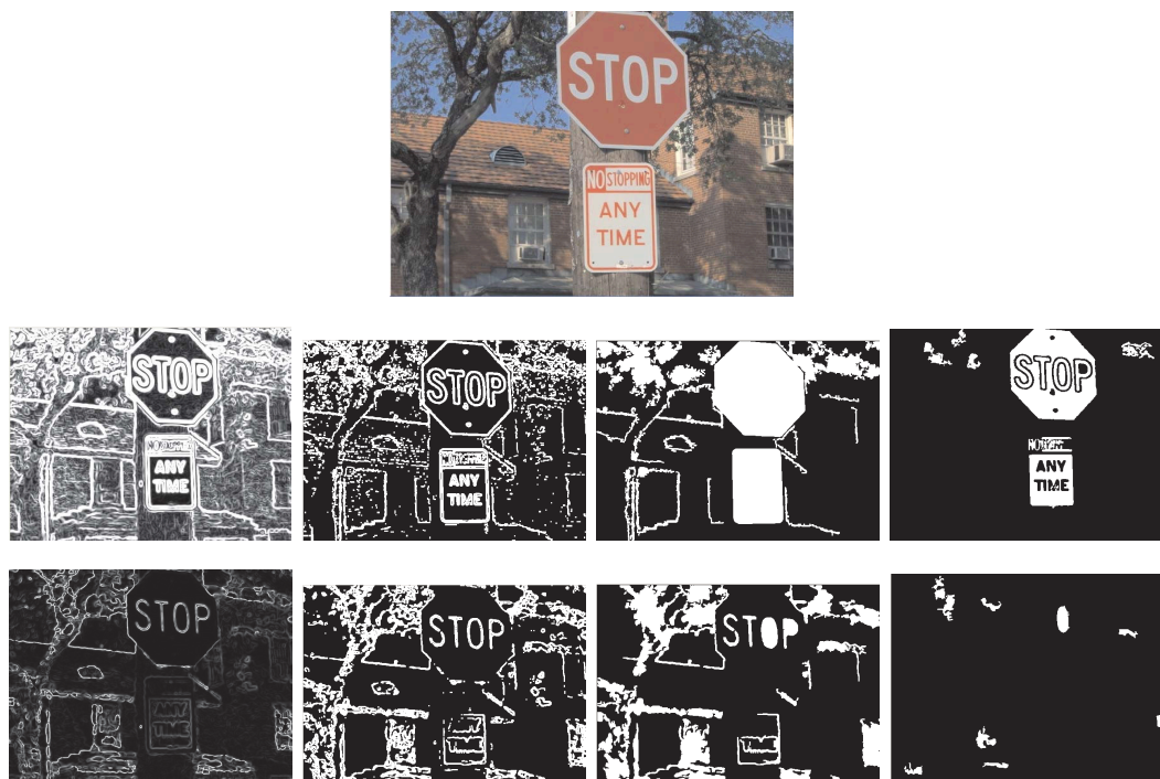
Fig. 5. An example of the whole process in locating signs. The first row is an input image. The second row shows sign localization process with our approach using chromatic edge segmentation. For comparison, we test with using Hue color segmentation. Results are shown in the last row. From left to right: chromatic edge images, binary edge images, filled images, final segmented images.
