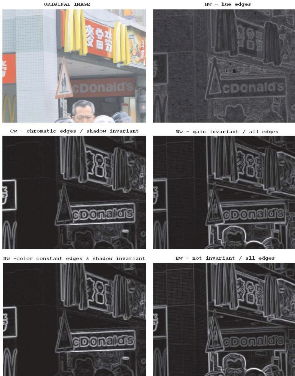
Fig. 2. An example of edge segmentation illustrating the discriminative power. Hue gives the worst segmentation (The input image is taken from [17]).
