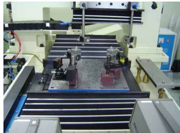
Fig. 3 Diagonal measurement in the XY plane
