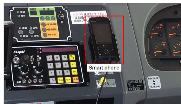
Fig. 6. Installed smart phone in a bus.
