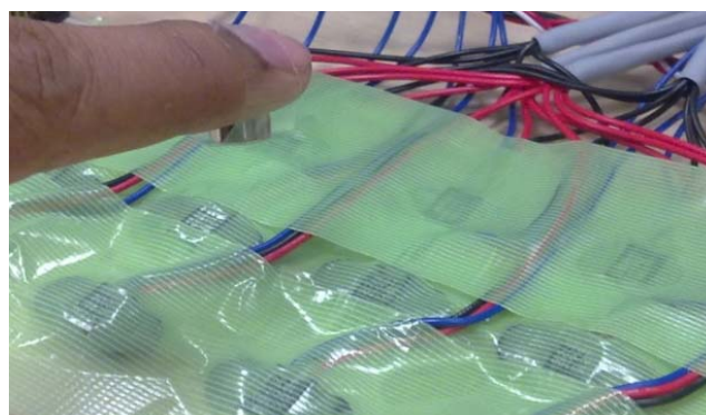
Fig. 1 User could freely move the neodymium magnet attached to the finger above the device surface and interact with the computer
