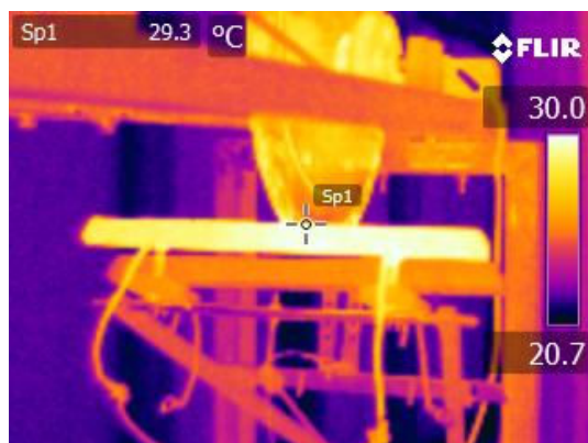
Fig. 15 Thermal spectrum of the sliding contact system for the test current of 8A, contact force of 10N and emissivity coefficient of 0.95 (different angle)
