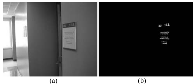
Fig. 12 Test result (a) Original Test Image (b) Text Extracted Image
