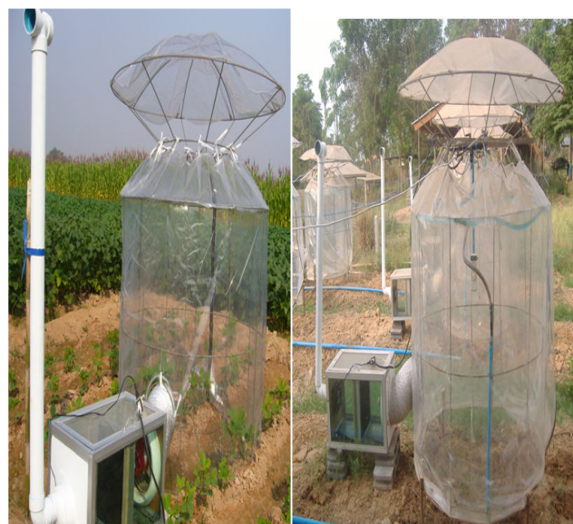
Fig. 2 Open top chamber in experiment with electrical control system
