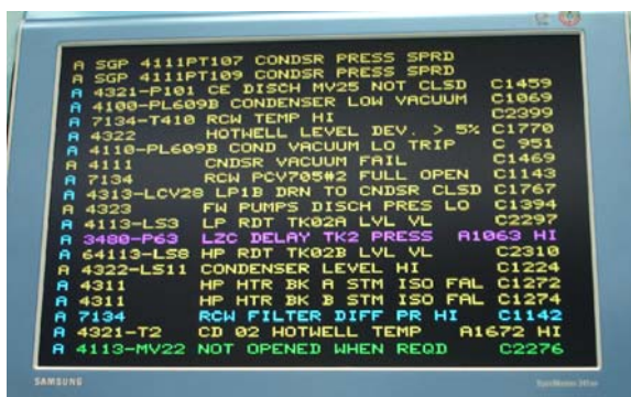
Fig. 11 A CRT alarm message display of an old NPP
