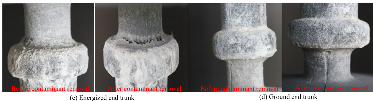
Fig. 6 Surface damaged straight shed specimen
