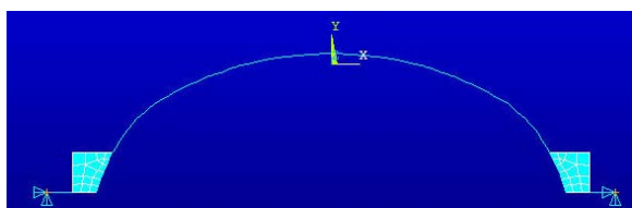
Fig. 2 2D Frame Analysis Model with Backing
