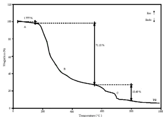
Fig. 6 TG curve of the as-synthesized LSCO precursor heated at 150 °C
