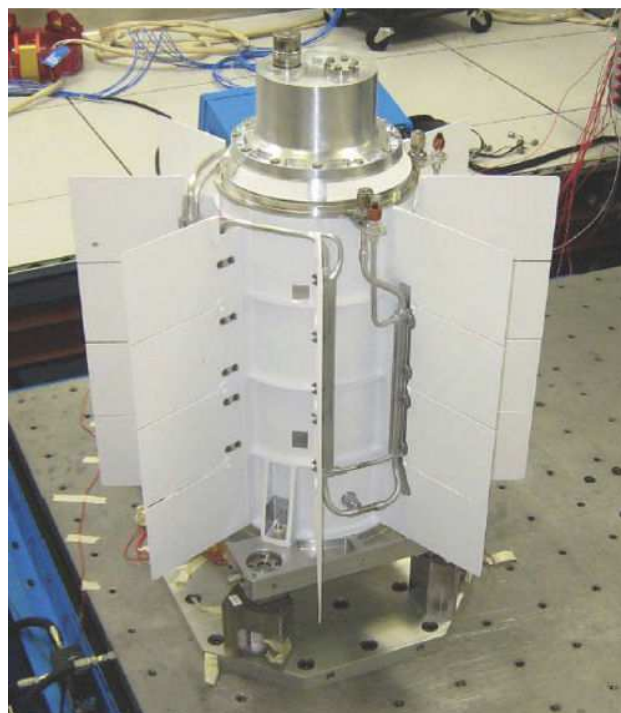
Fig. 5 View of the MMRTG (from: [15])
