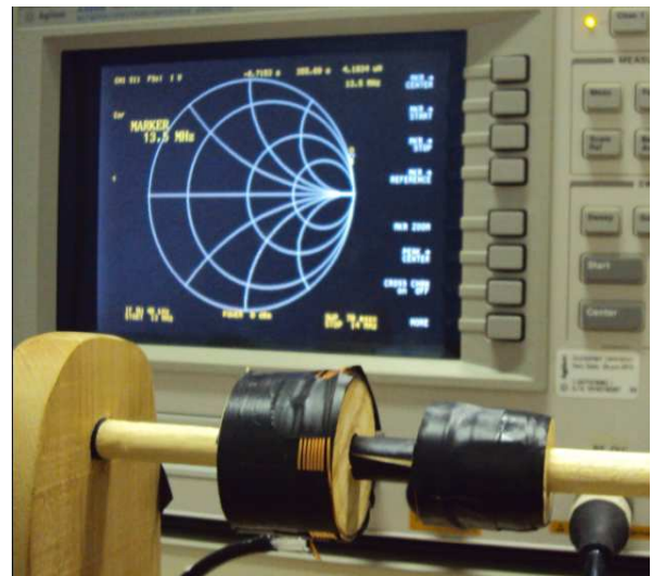
Fig. 7 Mutual inductance measurement
