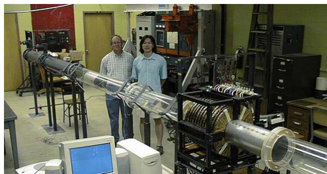
Fig. 1. The small-scale 8"-diameter PCP-TLIM system with the TLIM capsule pump located on the right. The TLIM stator has 12 slots and 4 poles.
