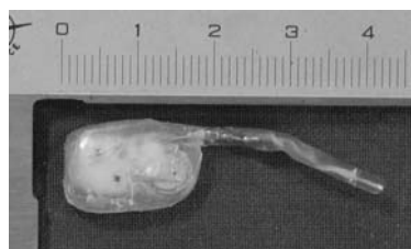
Fig. 2 The wireless intraoral pH telemeter
