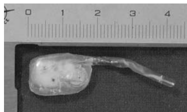
Fig. 2 The wireless intraoral pH telemeter
