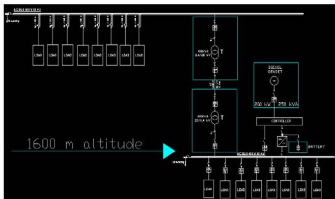
Fig. 4 1800 loads and 1600 m network diagram and loads
