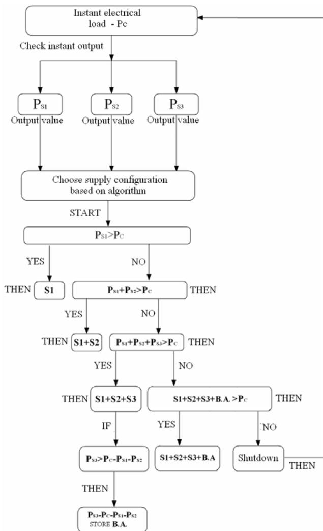
Fig. 6 Power flow management algorithm, electrical.
