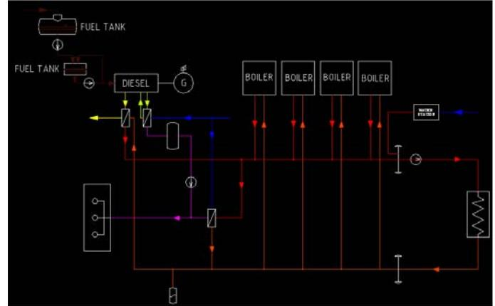
Fig. 5 Thermal diagram – 1800 m altitude (for 1600 m altitude there are only 3 boilers)
