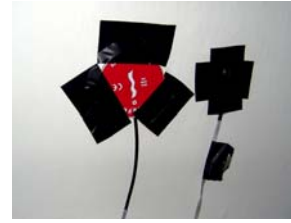
Fig. 5 Heat flux sensor and contact temperature probe
