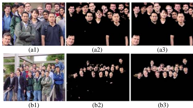
Fig. 7 (a1), (b1) are original photographs; (a2), (b2) are skin detection results; (a3), (b3) are final skin segmentation results
