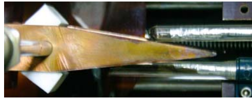
Fig. 9. Setup of induction probes in shifted configuration.
