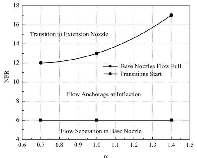
Fig. 6 Flow characteristics of the DBNs
