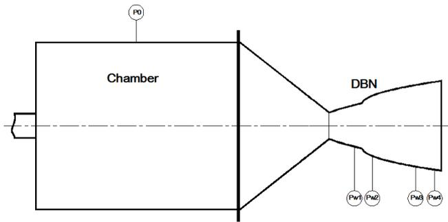
Fig. 3 Schematic of the test setup
