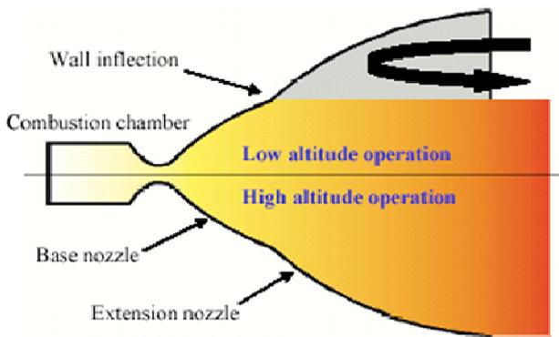
Fig. 1 Schematic of a DBN under the two modes of operation
