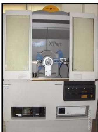
Fig. 2 Philips PANalytical XRD
