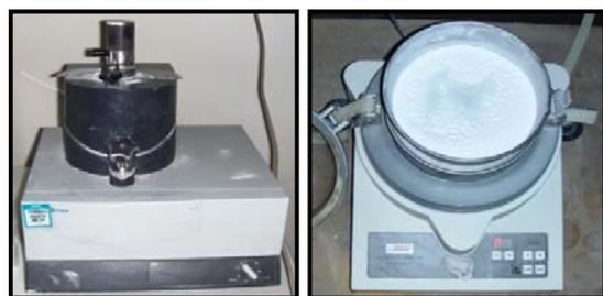
Fig. 1 (a) Grinding process, (b) Sieving process
