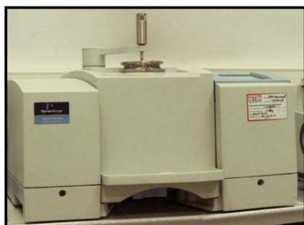
Fig. 3 Perkin Elmer Spectrum One FT-IR
