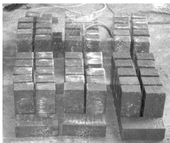
Fig.3 The curing of paving block samples
