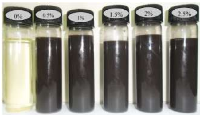
Fig. 1 Coconut oil based nanofluids of various concentrations
