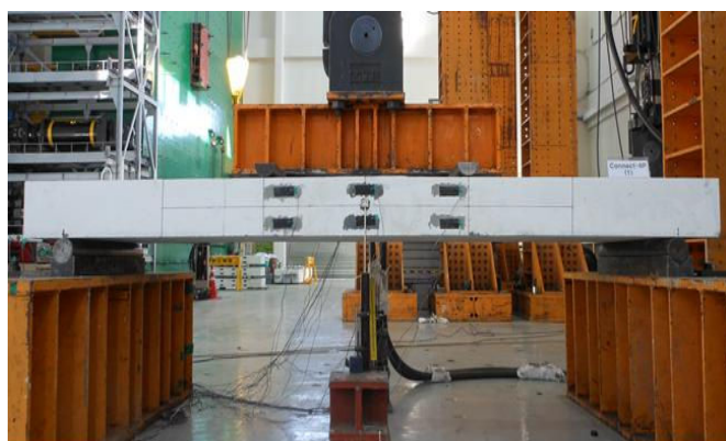
Fig. 5 Bending test setup
