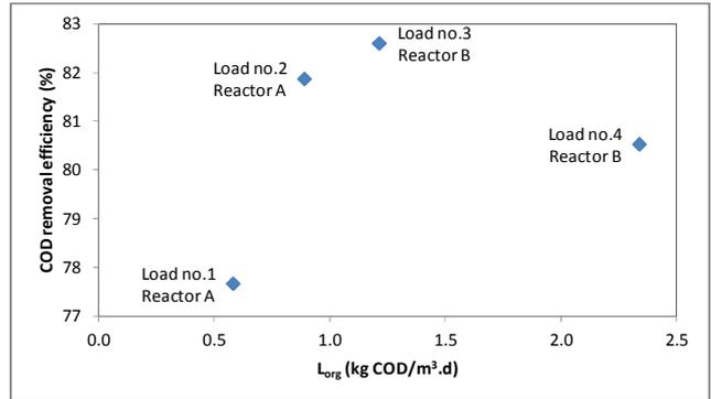
Fig. 5 COD removal efficiency percentage vs. volumetric organic loading rate applied.
