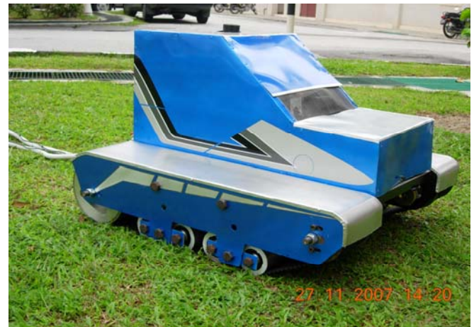
Fig. 6. Developed prototype of air-cushion track vehicle [9]
