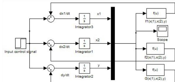
Fig. 14: Simulation structure diagram of the system (49).
