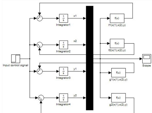
Fig. 1: Simulation structure diagram of the system (37).
