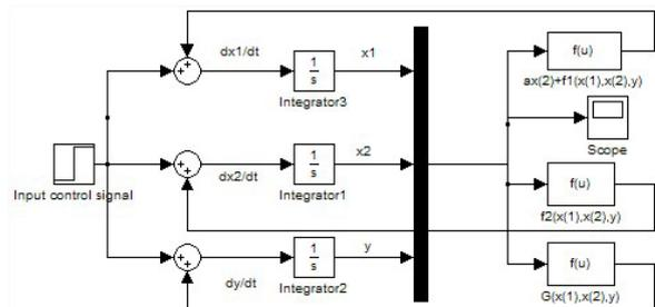
Fig. 11: Simulation structure diagram of the system (45).
