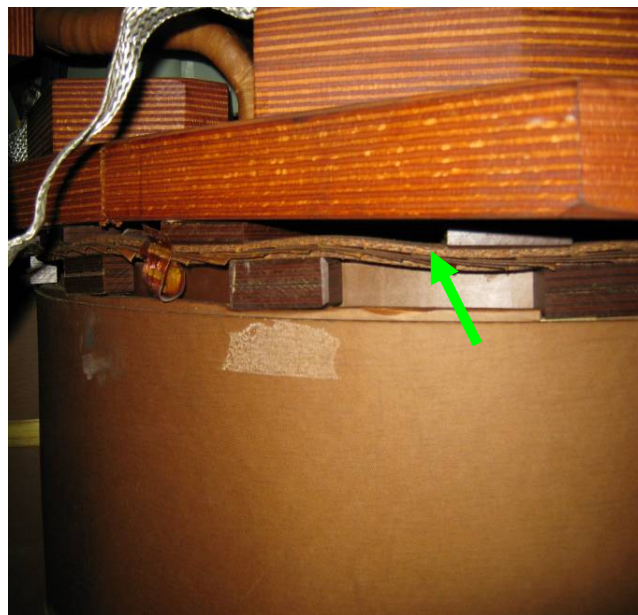
Fig. 8(a): Wavy pressboard due to coaxial force
