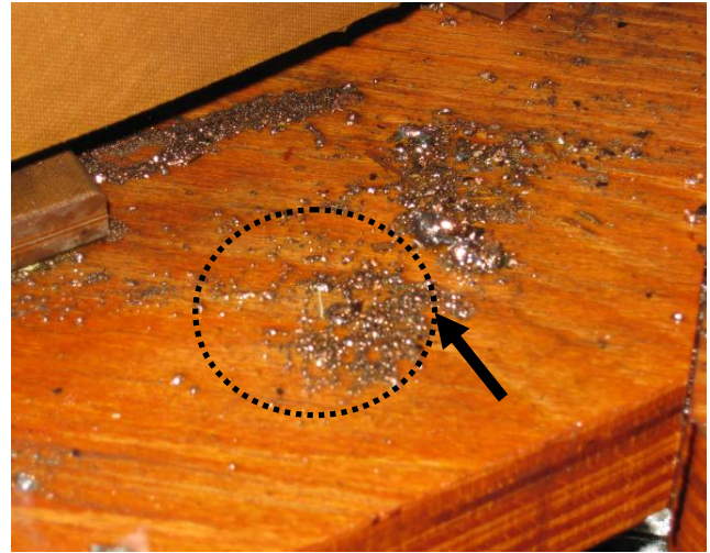
Fig. 11: Eroded copper chips
