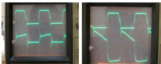
Fig. 8 a) V_{GS} and primary current of the transformer b) V_{GS} and the secondary output voltage of the transformer.
