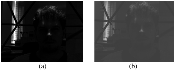
Fig. 9 Example of Yale_B illumination normalization image. (a) Example of the low light image, (b) illumination normalization result
