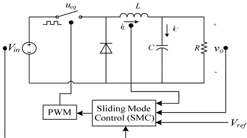
Fig. 1 Power system considered with SMC
