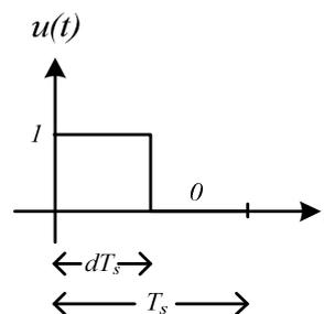
Fig. 2 The switching signal for the open-loop operation
