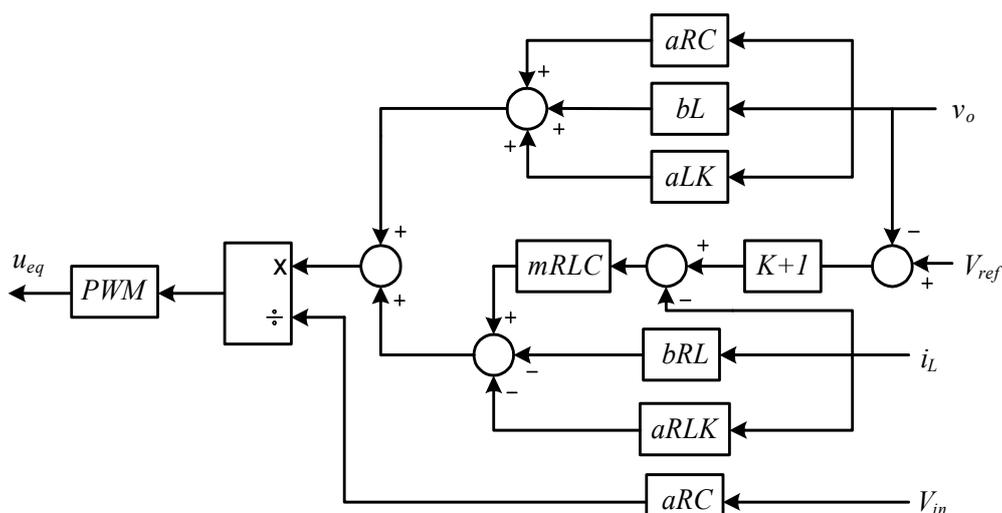
Fig. 3 The block diagram of  $u_{eq}$  calculation
