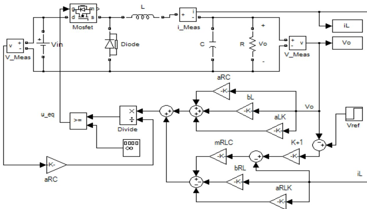
Fig. 4 The exact topology model of SPS<sup>TM</sup> in SIMULINK
