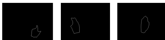
Fig. 3 Result of hand contour extraction algorithm
