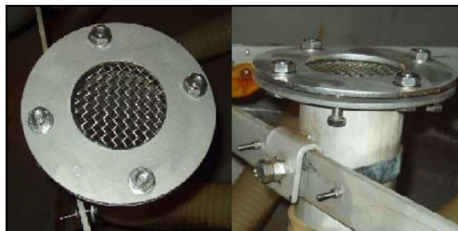
Fig. 8 Top and side view of nozzle with mesh installed
