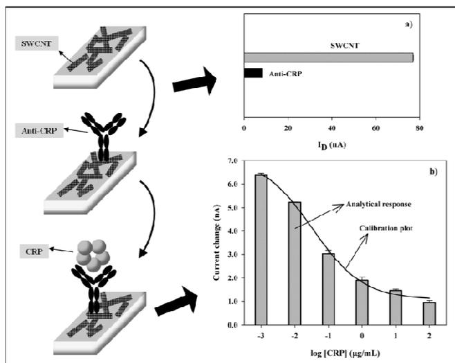
Fig. 3 Successive steps for the detection of CRP through interaction with their specific antibodies (anti-CRP) which were previously immobilized in NTFET surface; (a) Change in current before and after immobilization of anti-CRP; and (b) analytical response from the detection of CRP by NTFET devices and corresponding calibration model
