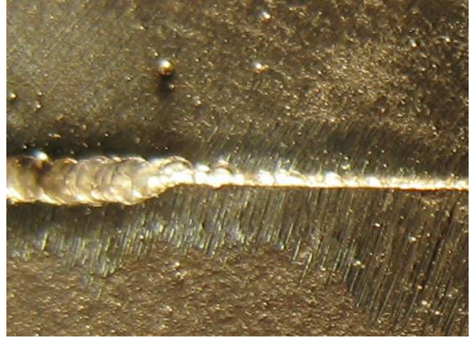
Fig. 4 Aspect of Ni-Cr alloy sample (welding with filler material): poor penetration on the opposite side
