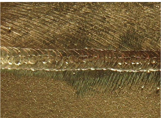
Fig. 3 Aspect of Ni-Cr alloy sample (welding without filler material): good penetration on the opposite side
