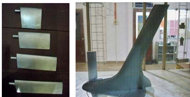
Fig. 2 Canards with different aspect ratio (left), BWB with canard (right)
