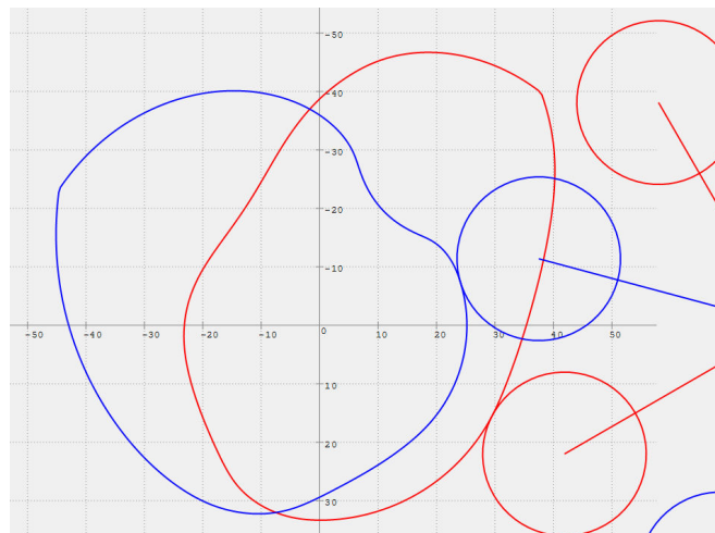
Fig. 6 Cam mechanism based on the unsymmetrical displacement diagram with unsymmetrical initial rotation of rollers
