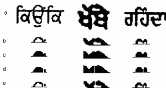
Fig. 18 a) example words, b) problem areas, c) top profile of problem areas, d) segmenting columns in top profiles, e) actual segmented characters
