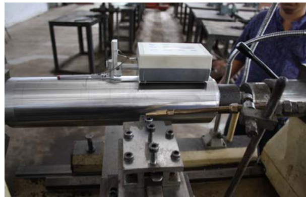
Fig.2 Photographic view of surface roughness measuring technique
