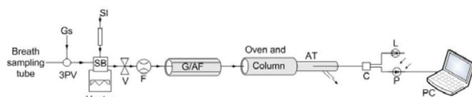
Fig. 1 Experimental configuration of the developed OF sensor for VOCs in standard and breath samples (Gs - carrier gas; 3PV - 3-port valve; SB - sampling bulb; SI - standards injection; V - valve; F - flow meter; G/AF - glass column/adsorbent fibers; AT - analytical tube; C - optical coupler; L - laser; P - photodetector; PC - personal computer)
