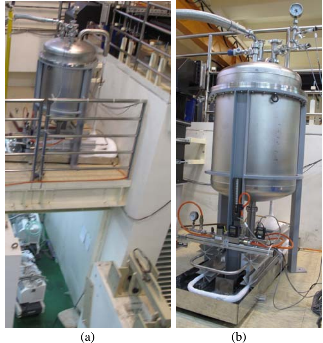
Fig. 4 Integrated with the passive and the flow control units, the buffer tank for vented nitrogen is located above the radiation-shielded area, in which the spare SRF module is cooled and tested
