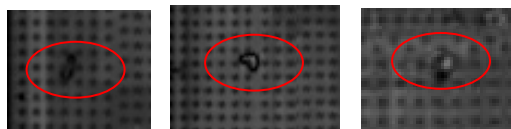
Not encompass two bumps Void in wafer Lot 1
