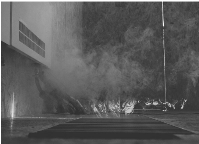
Fig. 4 Visualization of the flow structures at in- and outflow
