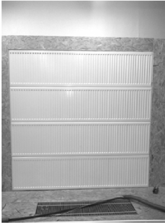
Fig. 3 Cooling wall and the measured convectors situated in the floor
