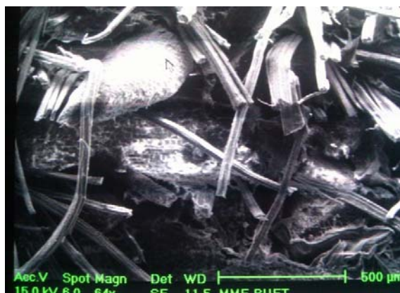
Fig. 13 Tensile fracture surface of 20% jute-coir fiber reinforced hybrid polypropylene composite
