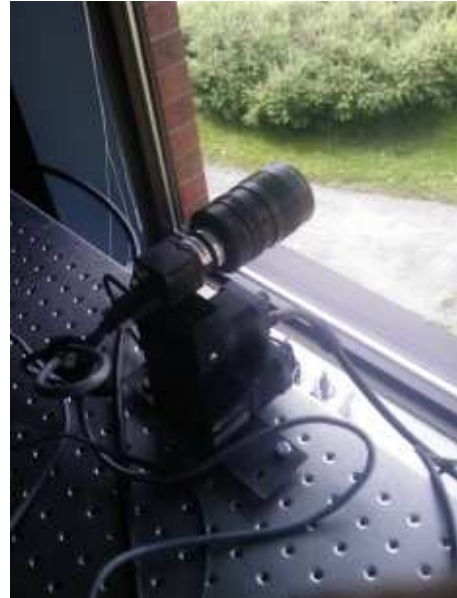
Fig. 6 Pan and Tilt unit PTU-D46-17with a 1024x768 camera
