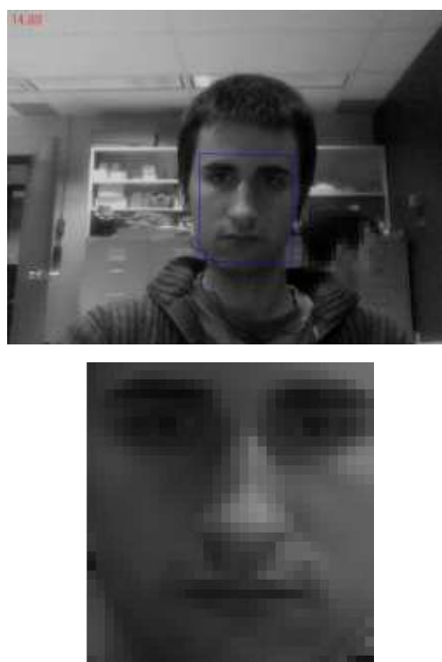
Fig. 4 Detected target in the image (upper image) and mean target image (lower image)
