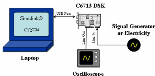
Fig. 3 Configuration for harmonic analyzer
