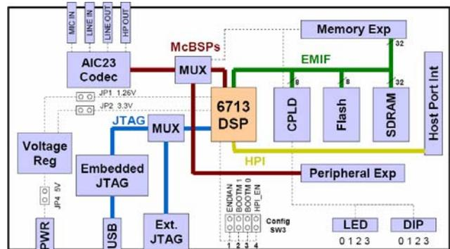
Fig. 1 Block diagram of TMS320C6713 DSK [11]
