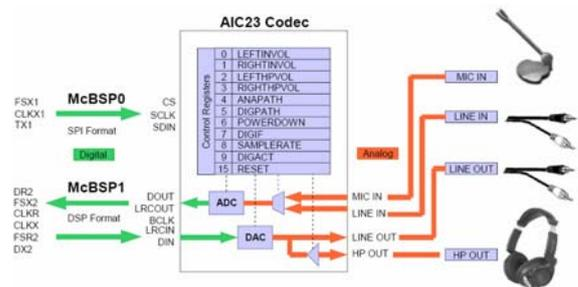
Fig. 2 Codec Interface of TMS320C6713 DSK [11]
