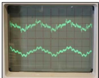
Fig. 6 Time domain plot of input (top) and output (bottom) of the DSK for circuit configuration in Fig. 5
