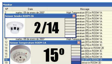
Fig. 8. Temperature Sensor, Smoke Sensor and Monitor Screens.
