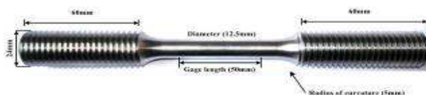
Fig. 2 Test specimen shape and dimension (KS B0801 10)
